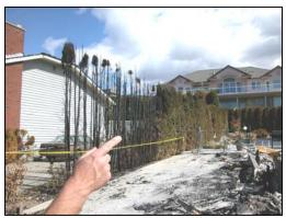
There are three priority zones for the modification of vegetation to reduce wildfire hazard. Priority Zone 1, the most important, is within 10 metres (30 feet) of the building. Without fuel modification in this critical area, the fire intensity and the rate of spread can make firefighting difficult or impossible.
