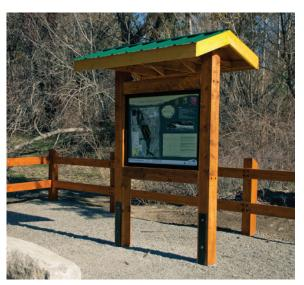
Timber kiosk with metal hardware and roof
