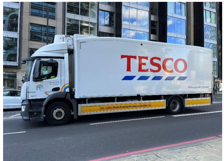
Figure ES-4: A goods movement vehicle with side underrun protection in the UK
